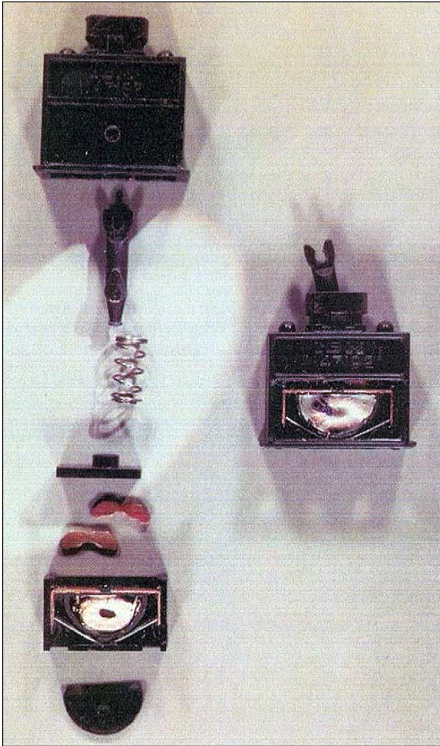
Exploded view of bugged power switch from a U.S. embassy typewriter
