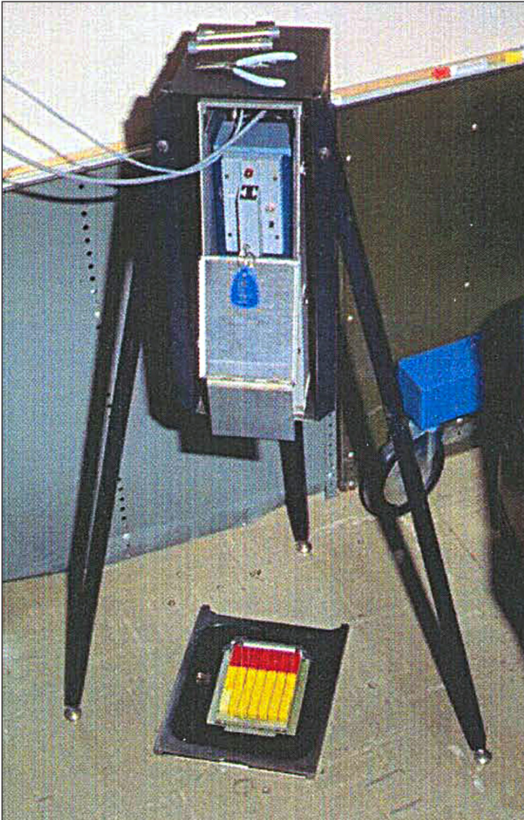
Primary x-ray machine used in detecting equipment bugs. This portable machine measured about 8 × 6 × 12-15 in. It was pointed at the floor when taking an x-ray; a sheet of x-ray film was placed under the item.
